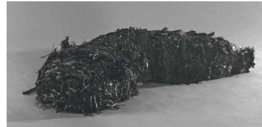
Material: carbon fibre, glass fibre, epoxy resin, latex binding agent
